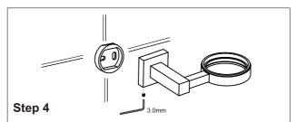
Slide the accessory onto the backing plate and tighten the set screw using Allen key provided.
