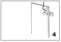
Fix the set screw on the knob, tighten it to avoid loose from fixing brackets.
