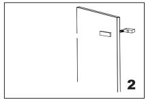
Add fixing bracket into the bolt, and tighten it with a small nut.
