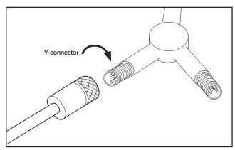
Connect the data cable to Y-connector.
