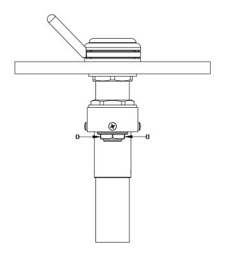
7. Tighten gear box bottom lock nut set screws. One or both set screws may be tightened.
