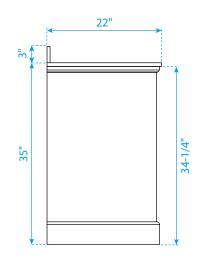
Note: Due to high probability of breakage, the backsplash comes in two pieces, cut from the same piece. All Measurements are ±1/4".
